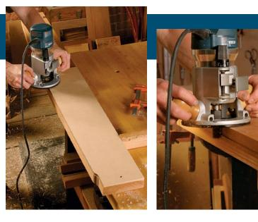
Thick stock requires a second pass. Remove the template and increase the bit depth. The bearing will now reference against the already trimmed surface of the workpiece.
