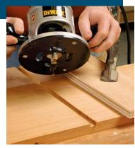
**Making the cut.** The router's base rides the edge of the jig. To ensure a straight cut, avoid rotating the base.
