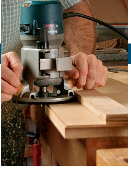
The guide keeps the router in line. Setup is easy, because the edge of the jig marks the edge of the cut.
