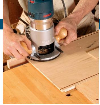
Keep the fence tight against the workpiece. This ensures that the cut is straight, smooth, and parallel to the edge.
