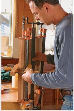
**Straighten a bowed panel.** Adjust the hand screw to span the pipe clamp and the panel. Tightening pulls the panel into a straight line. Check with a straightedge.
