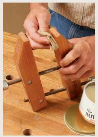
**Keep glue off your clamps.** A quick coat of wax on the clamping surface of the jaws will keep glue from sticking.
