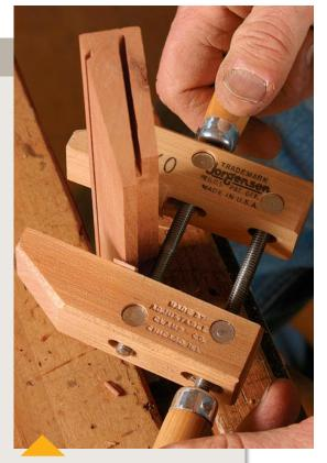
A positive grip, even on corners. The hand screw's light weight and precise adjustability make it great for repairs like this chipped-out edge.
