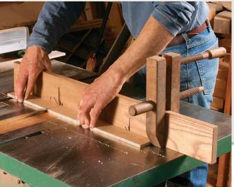
A simple stop block. A hand screw takes the place of a clamp-andblock setup for indexing repeated crosscuts.
