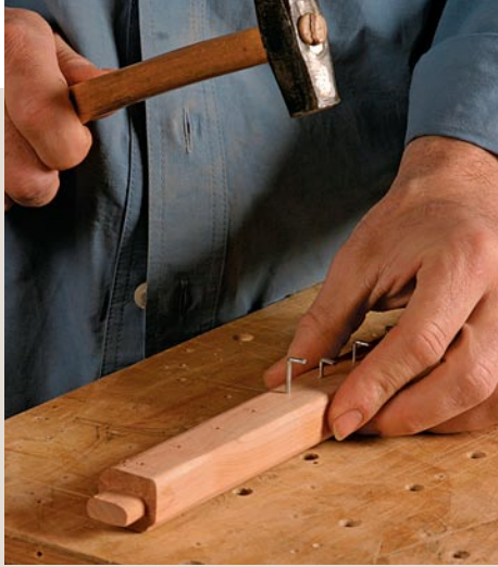
Attach the nails that hold the cord. Drill pilot holes along the seat-support rails and hammer the L-shaped nails in place.
