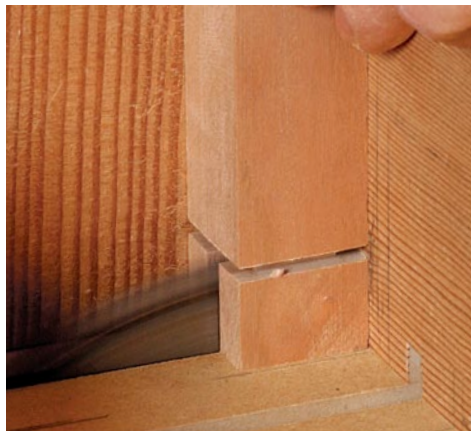
Begin in the middle on the double tenons. Once you've cut the shoulders, cut away the waste between the tenons in the middle of the stock (left). Cut the inside face of one tenon, then rotate the stock 180° for the second cut. Creep up on the right distance, using the leg to check the fit. Finally, cut the outside cheeks and ends (right).
