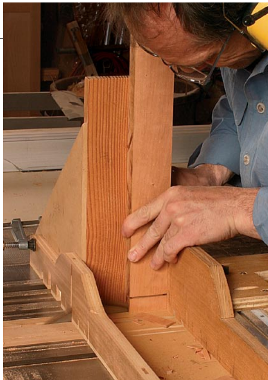
Add a tall fence to cut tenon cheeks. An auxiliary fence clamped to the sled supports the work when cutting the cheeks.
