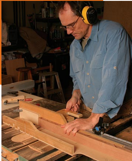
Cut tenon shoulders first. Edmundson uses a narrow, shopmade sled to cut the tenon shoulders, with a stop block clamped to it.
