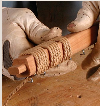
Wrap the long rails. Tack the cord to the end of the rail, then spin the rail to wind the cord. Wrap the cord five times between each nail, creating a gap at the nail that subsequent weaving will fill. Golf gloves reduce wear and tear on fingers.
