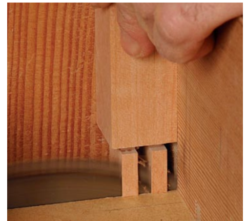
Begin in the middle on the double tenons. Once you've cut the shoulders, cut away the waste between the tenons in the middle of the stock (left). Cut the inside face of one tenon, then rotate the stock 180° for the second cut. Creep up on the right distance, using the leg to check the fit. Finally, cut the outside cheeks and ends (right).
