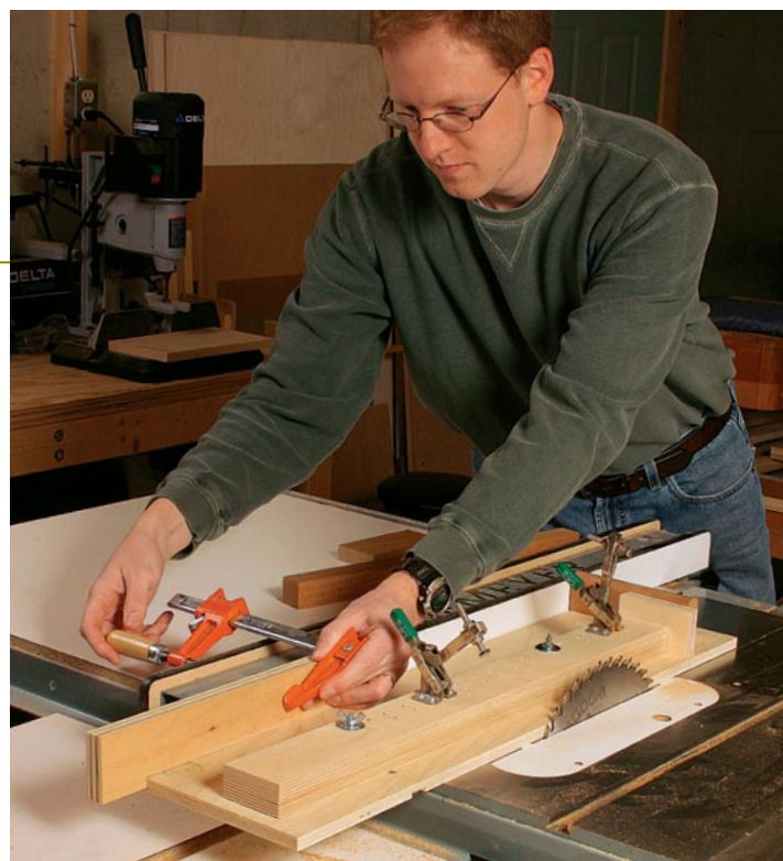
Set up a stopped cut. Clamp a hook-shaped stop to the fence so that you don't completely remove the waste from the long-taper cuts.
