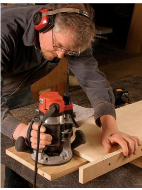
**Rout the slot.** Holding the router tight against the fence for control, cut until you reach the stop. Let the bit stop spinning before backing it out of the slot, or you could ruin the cut.
