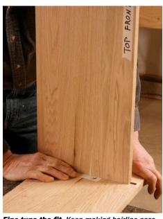
Fine-tune the fit. Keep making hairline passes on the router table to get the key to slide closer to home. To micro-adjust the fit, use a sanding block cut to the same angle as the dovetail bit and attach adhesive-backed P120-grit sandpaper to it (top). The goal is to get the shelf to slide with just hand pressure until it is about 1½ in. from being fully home (bottom).
