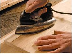
Shim out the bottom rear of the shelves. Use a shim of the same thickness used to taper the slots. Veneer tape is great because you can iron it on and take it off easily.
