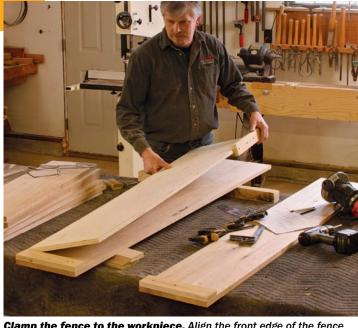
**Clamp the fence to the workpiece.** Align the front edge of the fence flush with the back of the case side and tight against the cleat at the top.
