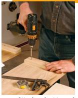
Attach a cleat to each case side. Screw the plywood cleat to the top of the inside case sides and perfectly square to the edges. Place screws in areas that will be wasted away when you profile the ends.
