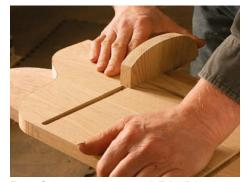
**Test piece gets you started.** Take light passes along both edges of a test piece, made from a shelf offcut, until it slides halfway or more into a slot with hand pressure.
