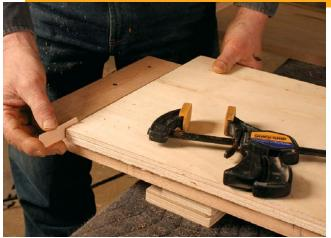
**Shim out the back side.** Place the shim between the fence and the cleat. Veneer tape is the perfect thickness (½32 in.) to create the desired taper.
