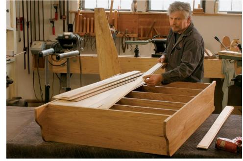
Nail in the back boards in order. Slide the top edges of the boards into the groove under the top shelf. To avoid misses, mark the shelf locations across the back, then nail each board to each shelf with 15-ga. finish nails.
