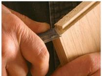
Trim 5/8 in. from the front of the kev. Use a handsaw to remove most of the waste, and clean up the cut with a sharp chisel.
