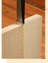
**GLUE FAILURE** A poor joint fails along the glueline.
