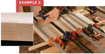
More pressure on maple. The effective glueline area is the same as for the pine (even though there are three boards to glue instead of two). The glue faces are quartersawn (see inset), so the recommended pressure is 600 psi. This total force of 9,900 lb. requires nine pipe clamps.
