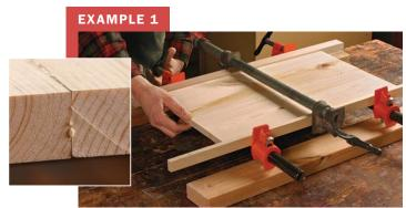
**Less pressure for pine.** These two pine boards have a glue surface area of 16½ sq. in. Because the glue faces are nearly flatsawn (see inset), the recommended pressure is 150 psi, requiring a total force of 2,475 lb. This can easily be met by using three ¾-in. pipe clamps.
