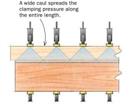
Where the glueline is close to the clamp head, place the clamps very close together or use a wide caul. Otherwise, some parts of the glueline will not receive sufficient pressure.
