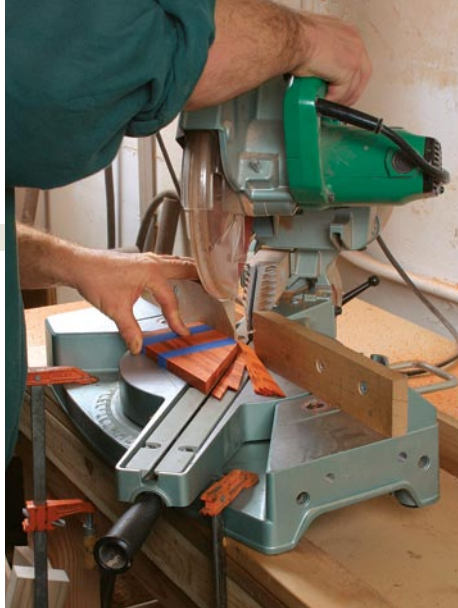
Leaves begin as simple shapes. Use a miter saw to cut blanks at a 45° angle from the end of a stack of veneers. Cut plenty of blanks, because you need 14 for each leaf.
