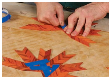
Glue groups of chevrons. Edge-glue seven chevrons to complete the leaf blank. Work carefully to be sure that all the chevron points converge at a single point.
