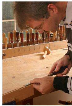
**Finish by hand.** Use a chisel to pare the rest of the sticking away.
