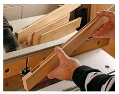
**Groove the rails and stiles.** Using a slotcutter, run the groove all the way through on the rails. But on the stiles, be sure to stop and start the groove in the mortise.
