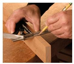
**Transfer the lines to the edges.** Use a square to bring the layout marks to the edges of the stiles.
