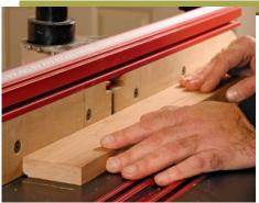
**Create the decorative profile.** Leaving the fence in place but adjusting the bit height, Bird makes two passes. The first scores the profile so the final cut can be made without tearout.
