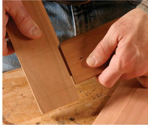
**Slide the rails and stiles together.** A beautiful fit depends on accurate layout, precise tablesaw setup, and careful chisel work.
