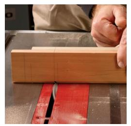
Use the reference line to make cuts. When mitering the stiles, match the reference mark on the backing board to the inside sticking line on the stile. To miter the rail stock, align the shoulder with the reference mark on the backing board.
