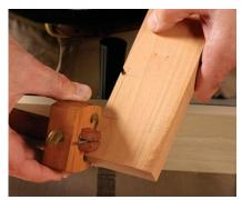
**Transfer the sticking line.** On the front of the stock, the profile is the reference, but you can use a marking gauge to scribe that line on the back of the stock.
