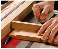
Use a dado set to cut the tenons. The miter gauge, in conjunction with a few graduated crosscuts ending at the rip fence, allows you to cut the cheek and establish the shoulder at the same time.
