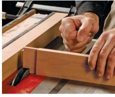
Complete the shoulder. Keeping the tablesaw fence in the same position, raise the blade and flip the stile on edge to cut the remainder of the shoulder.
