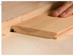
A straight bit cuts the tongue. Set the bit height to match the bottom of the groove.
