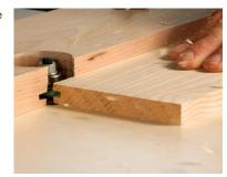
A slot cutter plows a groove.
