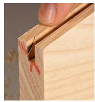
bead on the tongued section. When using thin stock, I don't bead the grooved edge because it will weaken the lip. This isn't an issue for larger cases with thicker back boards. If possible, set the top of the bead a little below the surface of the board so that it is not flattened during subsequent planing, scraping, and sanding stages.
