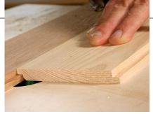
A shiplap fence simplifies the work. Allowing the stock to overlap the fence means both edges can be chamfered with one router-table setup.
