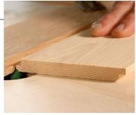
**Cut a chamfer on each edge.** Make sure that the profile doesn't compromise the integrity of the rabbet at either edge.
