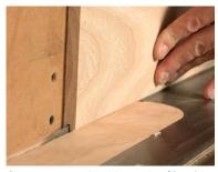
**Cut a groove.** A tablesaw kerf is wide enough to house a spline. The spline should be slightly narrower than the combined depth of the grooves to allow for movement.
