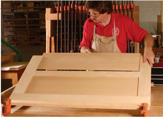
**Assemble the back.** The ½-in.- thick plywood is rabbeted on the back side, ensuring a good fit in the grooves. Check carefully once the clamps are on to make sure the assembly is flat, tapping the components into place with a deadblow hammer, if needed, as you tighten the clamps.
