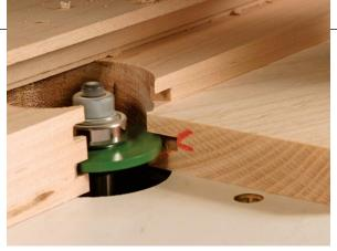
Cut a continuous groove in the frame members. On the stiles, the groove that houses the panel also serves as a mortise for the stub tenons on the rails. Because the cutter is buried into the fence, tearout is radically reduced. Make one pass in each direction to center the groove.
