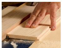
Matched rabbets form a joint. With the bit height set at half the thickness of the stock, all of the cuts can be made with one router-table setup.
