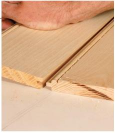
groove about ½ in. deep, so I bury the cutter in the fence to get a shallower cut and to reduce tearout. A fence-mounted feather-board adds both safety and accuracy.
