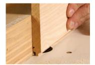
Cut the decorative element after cutting the joinery. Cutting the tongue first yields a cleaner cut because the beading bit isn't forced to hog away large amounts of waste material.
