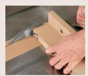
A similar test for crosscuts. Lay the boards flat to check the 90° stop on the miter gauge.
