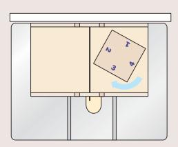
Make a test piece. Number the edges on a square of MDF. With edge 1 against the sled fence, trim each side in turn, rotating the piece clockwise between cuts.
