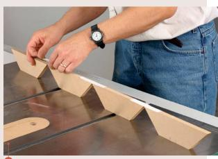
**2 Tape the corners.** This helps hold the pieces in place as you assemble the frame.
