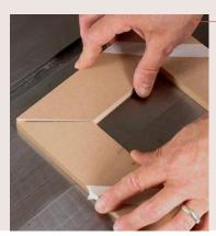
**Cook for the gap.** If the final corner doesn't fit snugly, it means the miter gauge isn't set at precisely 45° to the blade.
