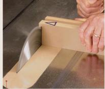
2 A test cut is more revealing. Use two pieces of lumber or medium-density fiberboard (MDF). Stand the pieces on edge and cut them in the same pass.
