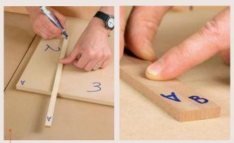
**(3)** Mark the ends of the strip. This identifies the front and back of the final cut. Make corresponding marks on the MDF square for future reference. Snap the final strip in two, lay the pieces on their sides, and compare the thickness of the two ends. Any variation means the crosscut sled's fence needs adjustment.
