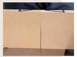
**3 The moment of truth.** Butt the two cut ends together. Any error will reveal itself as a tapered gap between the two ends.
