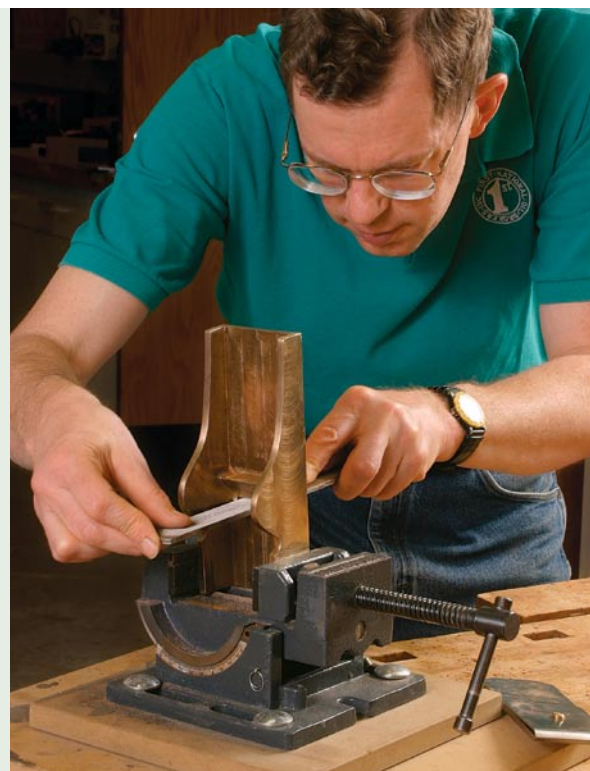
Opening the mouth. The mouth needs to be filed open very gradually until the blade just has clearance.
