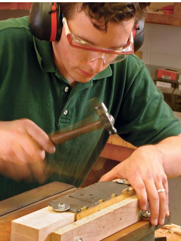
Pounding metal. Using a wooden jig resting on an improvised anvil, the author joins the dovetails together with a ball-peen hammer.
