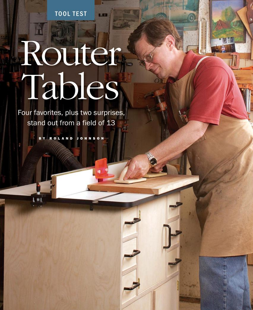
Retrools in the woodshop. Mounted in a table, the router becomes a mini-shaper that easily can make small moldings and joints, work with short stock, safely raise panels for doors, and pattern rout (shape wood using a template that rides along a bearing-guided bit). Most bit manufacturers recommend using large panel-raising bits or molding bits only in a table-mounted router because the bite a large bit takes makes it dangerous to use in a handheld router.
