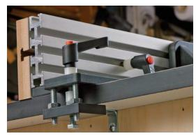
**T-tracks make for a versatile fence.** Commonly available T-track hardware can secure jigs to the Woodhaven fence in a number of spots.
