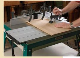
Sliding table carries the workpiece. Clamped by the miter gauge, this panel can be fed at an even rate for smoother cuts.
