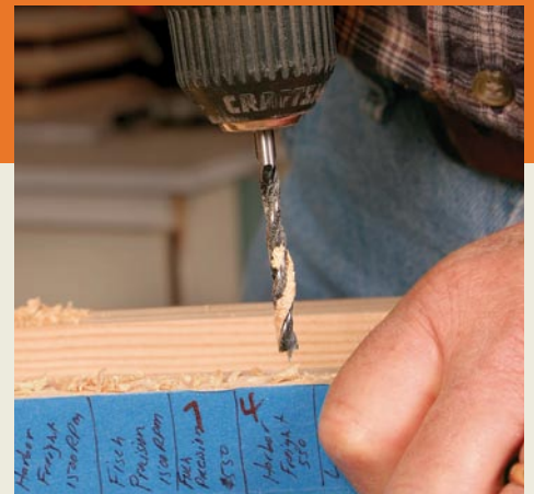
Clogged bits can't cut it. Some of the less-expensive bits were unable to clear the chips when drilling into pine.
