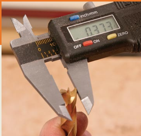
Checking the size. Minick used calipers to check the size of each bit as well as the diameter of the hole that it drilled to test for runout.
