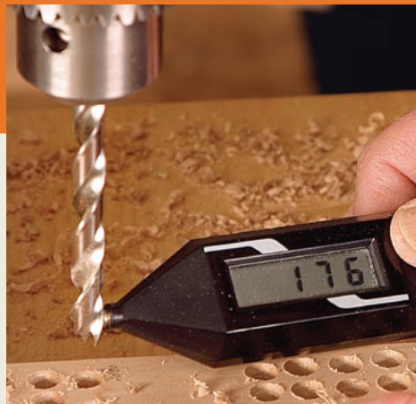
Drill bits get hot. A temperature probe measured how hot the bits got when drilling into hard maple. Well-designed bits stayed coolest.
