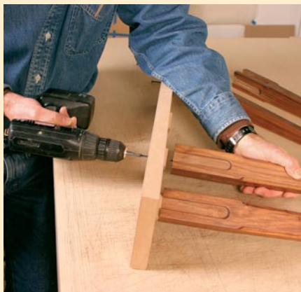
Finishing board for legs. To hold legs vertical while being finished, screw the tops to a piece of MDF. Keep one corner pointed forward so that you have access to two sides of the leg at a time.
