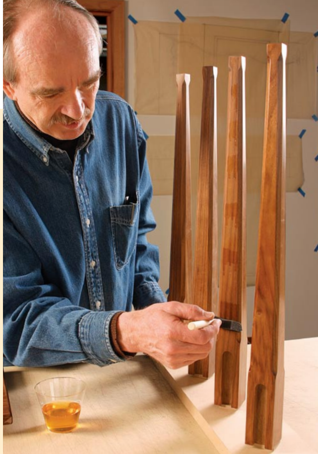
Pre-deposit finish on vertical surfaces, too. Deposit finish working from top to bottom, then apply a continuous stroke in the reverse direction (left).
