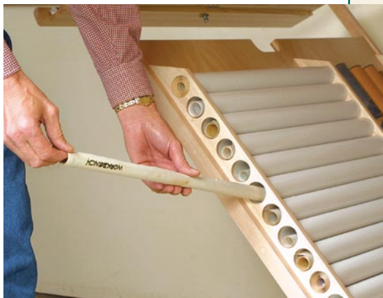
A place to store finished drawings. Completed drawings can be rolled up and stored in PVC tubes mounted behind the support panel.
