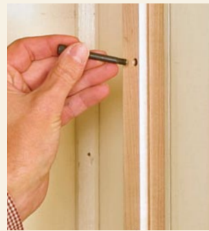
Screw stops. Fillister-head screws, slipped into matching holes in each of the frame sides, act as pegs for the bearings to rest on and establish the position of the table.
