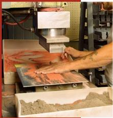
bination stone. A mixture of 100-grit abrasive and ceramic material is used to fill the hollow area in the molding table (top). After the layer of coarse grit has been compressed at nearly 2,500 psi, a layer of 320-grit mixture is spread over the top (center). After a second compressing, the combination stone joins others ready to be baked for about 48 hours in a kiln at 2,000°F (right).
