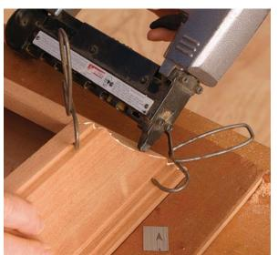
Use specialized clamps. Apply a spring clamp to the outer joint of the molding, massage the joint to find the best fit, and then apply a second clamp (above). To make the joint stronger, use 23-ga., headless pin nails to reinforce both sides of the joint (left). The holes are easily filled with dust when the molding is lightly sanded.
