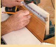
Use the fence to measure outside corners. On a piece with two outside corners, it is impossible to hook the tape measure over the end. Instead, align the molding with the square end of the auxiliary fence and hook the tape measure to the fence.
