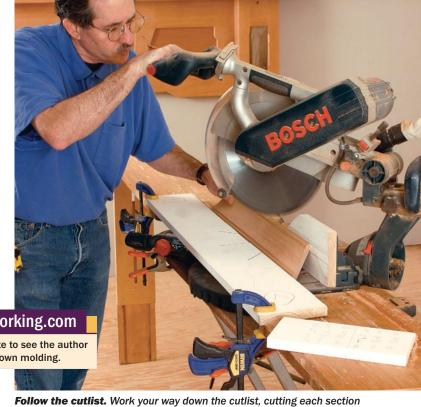
**Follow the cutlist.** Work your way down the cutlist, cutting each section of molding to the prescribed length and with the correct miter at each end.
