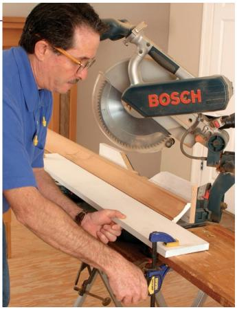
piece of molding at its base. On either side of the number I write the type of cut required. I indicate inside corners with a "V," for outside corners I write "OC," and for 90° cuts I write a "B" (butt joint).
