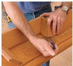
Clamp inside corners. To give the spring clamps a better grip on the smooth back of an inside corner, drill small holes 1/8 in. deep.
