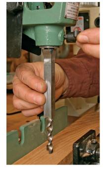
the shank and the bushing (top photo). To help wood chips eject as easily as possible when you're cutting a mortise, position the slot of the chisel so that it faces either left or right.
