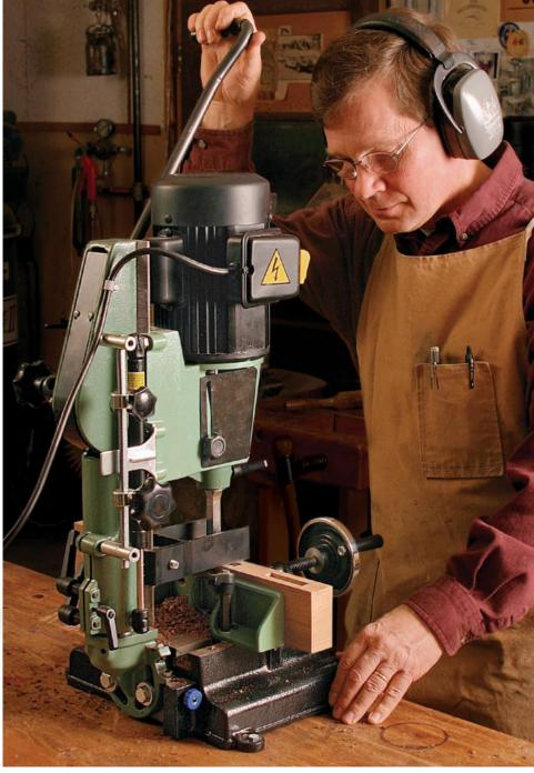
hen it comes to cutting mortises, there is no shortage of ways to get the job done. One of the most efficient is to use a mortising machine, also called a hollow-chisel mortiser. Properly set up and operated, it cuts straight, square-sided mortises in relatively short order.
