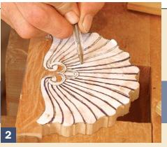
**Trace the shell.** With a ballpoint pen, draw over the lines defining the rays of the shell. The pressure will create faint lines in the wood, visible when the template is peeled away.
