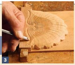
**Form the convex profile.** First establish the basic convex shape of the shell, redraw the lines of the rays, and then relieve the base of the shell.
