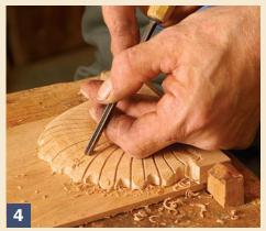
**Define the rays of the shell.** Use a V-parting tool to create the veins that divide the convex and concave rays of the shell.
