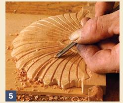
**Form the concave rays.** Use both V-parting tools and sweep gouges to carve the concave rays first.
