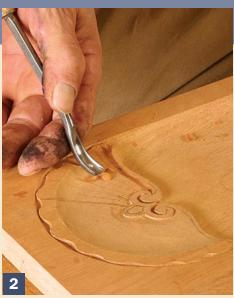
**Carve the concave shell.** As with the convex shell, first establish the perimeter profile, then the fleur-de-lis. Establish the main profile, and finally create the rays. Spoon gouges work well in the concave sections.
