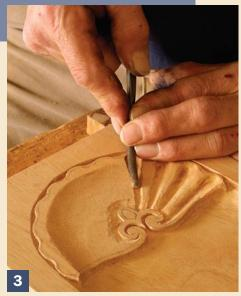
**Alternative shaping tools are useful.** In difficult grain or confined locations, files, rasps, and rifflers come in handy.
