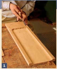
**Shape the cabinet door.** Use a router to remove the bulk of the wood from the recessed center of the door and gouges to create the curves. Use a V-parting tool to define the edge of the shell.
