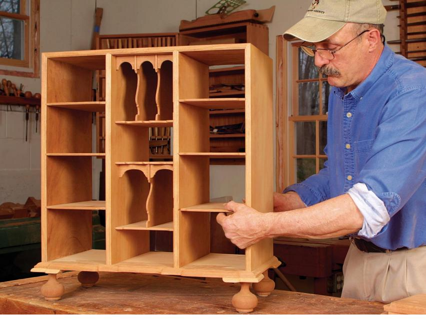
vertical dividers in the center compartment have a birdlike profile. The dividers fit in <sup>1</sup>/<sub>8</sub>-in.-deep by <sup>1</sup>/<sub>4</sub>-in.-wide dadoes.
