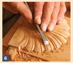
**Round over the convex rays.** An inverted fishtail gouge works well to establish the convex rays.
