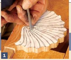
**Carve with a template.** Spray-mount the convex shell design to the carving blank. Bandsaw and carve the edge profile and then define the fleur-de-lis with carving tools.
