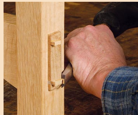
Drive and trim the wedges. During glue-up, drive in the two wedges evenly (top) to ensure proper assembly. After the glue has set, use a chisel to trim the wedges flush with the beveled ends (bottom). Use sandpaper to clean up the surface, including any glue residue.
