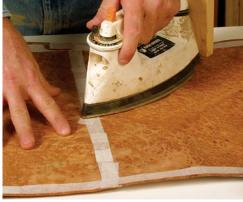
Tape the leaves together. Temporarily join the leaves with blue masking tape, then apply veneer tape (left), over the seam. Tear away the masking tape, and use more veneer tape to fill the gaps. Iron the veneer tape immediately to release the moisture (right).
