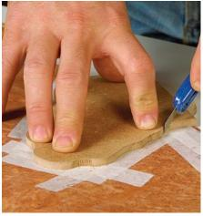
Template guides the cut. To prevent checking, tape the veneer around the area to be cut, then make several passes with your cutter.
