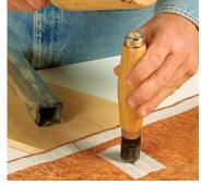
A cloud-shaped punch is best for burl. This type of punch is commercially available or can be made by hand from steel pipe.
