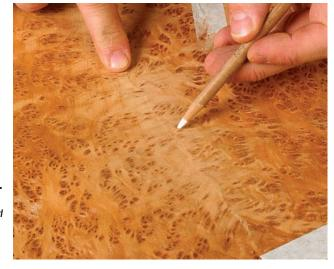
Flip the leaves to inspect the seam. The irregular seam blends with the burl and will be hard to locate after finish has been applied.
