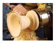
Establish the outside shape. Use a detailing or bowl gouge to form the profile of the turning, always cutting in a downhill direction and with the grain.
