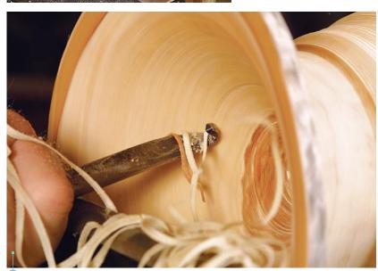
Continue the roughing and smoothing process. Use a bowl gouge to remove material quickly, then a ring or hook tool to smooth out the final surfaces
