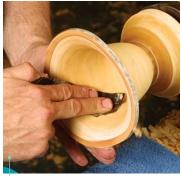
Wet-sand on the lathe. Small turnings can be sanded on the lathe, using water and wet-or-dry abrasives ranging from 120 grit to 320 grit.
