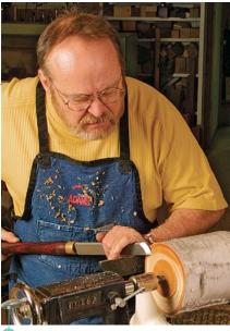
Face off the top with a skew chisel. A shoulder cut with a skew chisel will make a cleaner cut in the bark than a parting tool.
