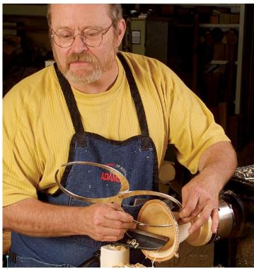
Measure the wall thickness. Aim for consistently thick walls to prevent the wood from cracking as it dries.
