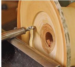
Switch to a ring tool or hook tool. Smooth the surface left by the gouge with either the ring tool (left) or hook tool (below). Cut from the center to the rim to produce a smooth surface. Hold the tool so that the flute is pointing between 9 and 10 o'clock.
