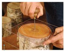
Find the center. Lacer uses a clear plastic template with various diameters traced on it to help locate the center of the log.
