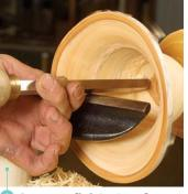
Scrape a finished surface. A rounded scraper tilted to 45° generates a shear cut, which reduces sanding time.
