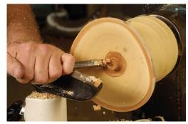
Rough out the inside rim with a bowl gouge. This may cause tearout, but it is effective at removing waste quickly.
