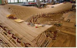
**Steaming the stringers.** Pliessnig steams and bends the stringers one by one, clamping them in place overnight. Then he'll remove one, sand it, and glue it in place with epoxy. For extra strength, he makes every third or fourth rib thicker.
