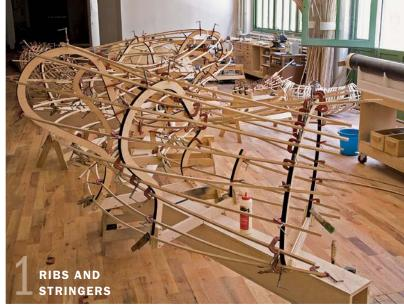
**Sketching the structure.** Pliessnig roughs out the sofa's form with temporary ribs and stringers. The ribs, jigsawn or CNC laser-cut from plywood, are fixed to a plywood strongback that snakes along the centerline of the piece providing a level surface. The temporary "sketching stringers," steam-bent from white oak, let him "play with the shape to make it more attractive or more usable."
