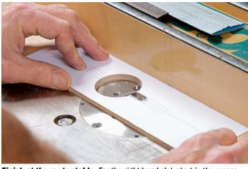
**Finish at the router table.** For the right-hand slot, start in the recess (above). But to keep the router action working in your favor, start the lefthand slot with a plunge cut at the end, and rout toward the recess (right). Mark the table's fence to know where to start this blind cut.
