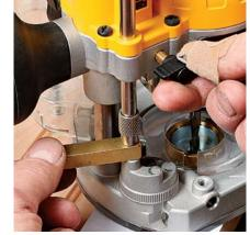
**Set the depth.** With the template clamped in place, lower the bit against the workpiece. Then set the depth stop, using a spacer equal to the desired depth of cut.
