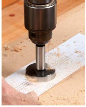
**Cut the recess first.** Hubel generates most of his pull designs in a CAD program, and glues a printout to <sup>1</sup>/<sub>4</sub>-in. MDF (left). With pulls with a round recess, Hubel drills the template (above), but for ovals and other designs, he uses the scrollsaw, and sands the opening smooth.
