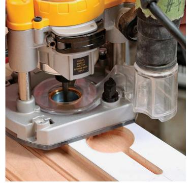
**Almost foolproof.** Use dust collection if possible. Start at the end of one slot and move into the middle of the recess. From there work outward, cutting in a counterclockwise circular path. To avoid burn marks at the edge of the recess, leave a whisker of material there for a final pass. Then finish the other slot.
