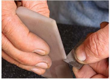
**Get inside.** To hone the concave area of the scraper, Hack uses a slip stone (above). You can substitute a rounded stick or dowel and fine sandpaper (right) to do the same job.
