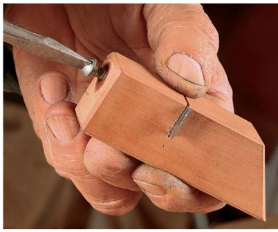
**Cure for a fat kerf.** If the scraper is loose in the kerf, drill and install a screw or bolt to wedge it in place.
