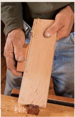
**Colored pencil** guides the way. Mark the apex of the bead (or the high point of a different profile) on the edge of the board (above left) and adjust the scraper so that its tooth is just beyond that mark (above right). Cut until the pencil line just disappears. This will create a bead that's parallel to the original surface. Remove any fuzz with fine sandpaper (below).
