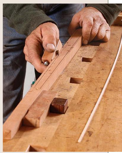
Works as an inlay tool. Hack uses scratch stocks to excavate for string inlay. The scraper is filed with a tooth profile to match the width of the stringing.
