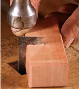
Install the scraper. Tap in the scraper until it bottoms out in the kerf (above). Then adjust its projection (left) from the block to locate the bead (or other profile) perfectly on the work. Test it on scrap until you have the location nailed.
