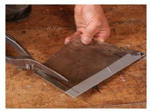
**Snip.** Cut out the scraper blank from a piece of spring temper steel. Hack takes it from an old handsaw blade. The size will vary based on the profile you're trying to achieve, but for a simple bead a blank 1 in. by 1½ in. is good.
