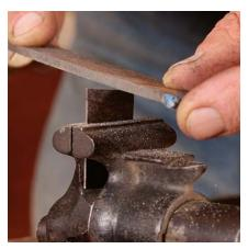
**Smooth.** Use a flat mill file to square up the edges. Hack holds the scraper in a small machinist vise but lacking that, you can use a bench vise.
