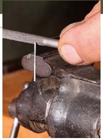
**Shape.** A bead profile is a great starting point for getting into scratch stocks. To create the profile Hack uses a round chainsaw file.
