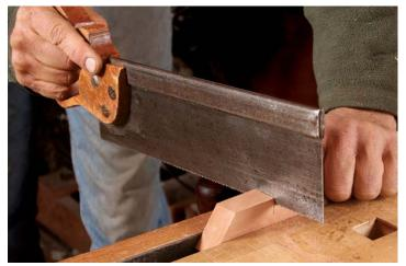
**Cut a kerf.** Size the holder to fit your grip— $\frac{7}{8}$  in. thick by  $1\frac{1}{4}$  in. wide by  $3\frac{1}{2}$  in. long is a good starting point. Smooth its surfaces and chamfer the edges, then cut a kerf for the scraper.
