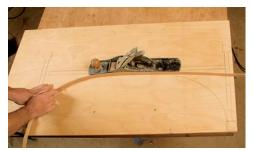
Lay out the curve on the drawing. Use a flexible batten to create a curve that gets tighter near its ends. Trace the shape on your drawing to be sure the curve hits the right spots. Use that curve to make a lamination form.
