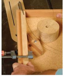
**Cut the parts one at a time.** Cam-action disks clamp the curved part in place (left); the side stretcher simply is clamped to the fence (right). After cutting one joint, just flip the curved stretcher and repeat the process at the other end.
