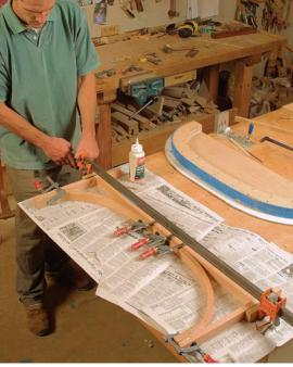
Glue up the whole assembly at once. Make curved clamp pads for the inside faces of the splice joints. The pins keep the splice joints from slipping.
