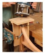
Router jig for floatingtenon joinery. To cut a precise mortise in one end of the finished assembly, make a jig to secure the workpiece and act as a router template.
