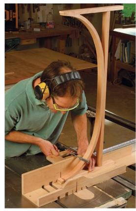
Trim the assembly to final size. Lay the stretcher assembly on the drawing to mark the final length of the front ends. and cut them with a crosscutting sled on the tablesaw. Then measure from the front ends to mark and cut the back ends.
