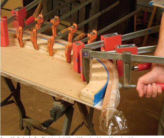
Assemble the lamination. Start clamping at the middle and work toward the ends, using a clamping caul made from five or six strips of 1/16-in.-thick birch plywood to prevent bumps.
