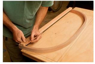
Trim the ends. Again, use the drawing as a guide. Mark and trim each end 1 in. extralong at this point. Use a long stick to ensure that the cuts will be aligned.
