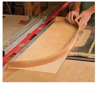
Flatten the back for a strong glue joint. To keep the workpiece stable during the cut, tape or clamp it to a plywood base.
