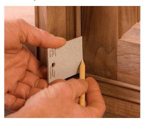
**1. Mark the latch side for trimming.** Press the door against the hinge side, setting it inside the case slightly. Use two shims to lay out the opposite side. Trim this edge on the jointer to within 1/32 in. of the marks to allow for discrepancies that may occur when hanging the door.
