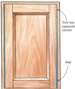
also might help the door slip all the way into the opening, if it won't do so already. It is critical that you don't trim too much off the bottom edge: Aim for eliminating only one-half to two-thirds of the gap. Later you'll eliminate the remainder by trimming the hinge side of the door, thereby not taking too much off any one edge.
