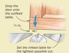
Starting point. With the jointer running, place the corner of the door to be trimmed onto the infeed table. Lower the opposite corner with about 1/2 in. overlapping the outfeed table.
