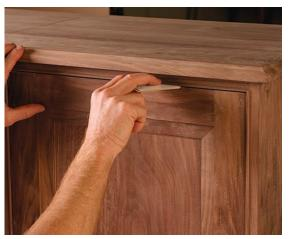
3. After trimming on the tablesaw, return the door to the opening. Don't place any shims underneath the door. To check both the top and bottom gaps at once, slide two shims in the gap along the top edge.
