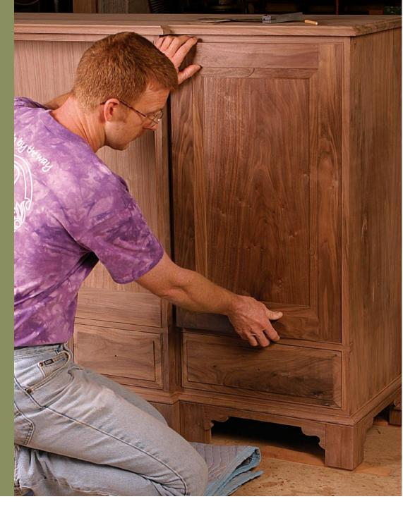
ver the years I've had to hang hundreds of inset cabinet doors. In that time, I have refined an efficient process for fitting them accurately to their openings. The method works for most styles of furniture and cabinetry.
