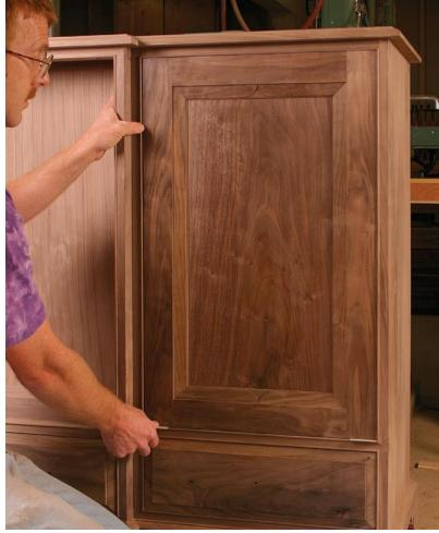
1. Place the door on shims. With one shim at each bottom corner, push the door inward about 1/8 in. to prepare for the next step. The door probably will balance in this position.
