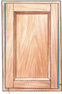
Remove a portion of the gap on the hinge side by making a tapered cut along the bottom of the door.
