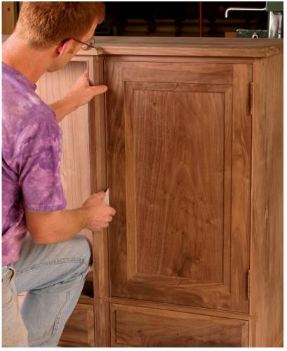
**3. One last step.** After the door has been hung, slide a shim along the latch side to recheck your layout marks. Make the final trimming cuts on the jointer.
