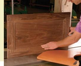
Making the cut. Push the door through as you would for an ordinary cut. If there is enough material left, make a normal pass to clean up the edge.
