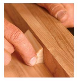
need for clamps. I use yellow glue because it is strong, grabs quickly, and allows a tiny bit of creep or movement. I try to orient the grain of the block in the same direction as the grain of the wood to which it's attached, but sometimes one face of the block will be joined across the grain. In these cases, glue with a little flexibility is useful.
