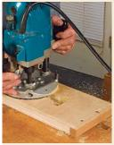
Hidden bolt. Use a jig to rout a T-shaped slot inside the side rails (above). Then insert the bolt and tighten it into the nut embedded in the head or foot rail (right).
