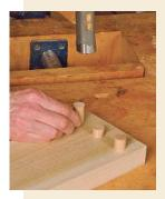
Install the clip plate. Glue hardwood dowels into the inside of the side rail to give the screws something to bite into besides end grain.
