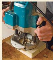
A recess for the nut. Use a plunge router and a straight bit to cut a mortise on the inside of the rail.
