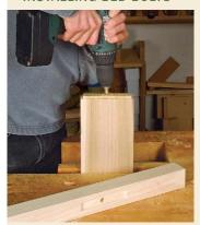
**Drill the bolt hole.** After drilling through the post into the tenon, remove the post and complete the hole to its full depth.
