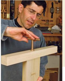
One tight joint. After cutting the tenon flush with the rail, insert the bolt through the post and crank it tight with the bedbolt wrench.
