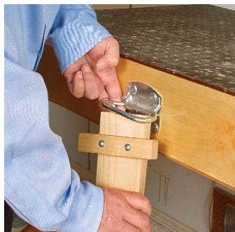
Handle doubles as leg connector. The handle not only is used to lift and lower the table, but it also connects the leg to the table.
