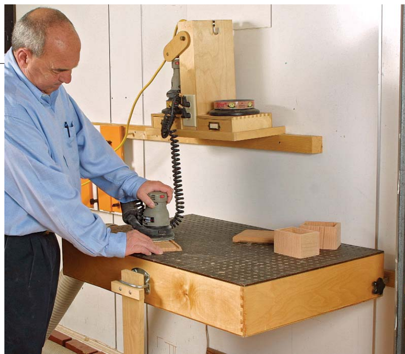
Handle doubles as leg connector. The handle not only is used to lift and lower the table, but it also connects the leg to the table.
