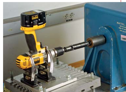
Testing torque. Peter Sawchuck, an engineer with Consumers Union, measured torque at a lab in Yonkers, N.Y. (left). Each drill was mounted in a dynamometer (above) to measure power.
