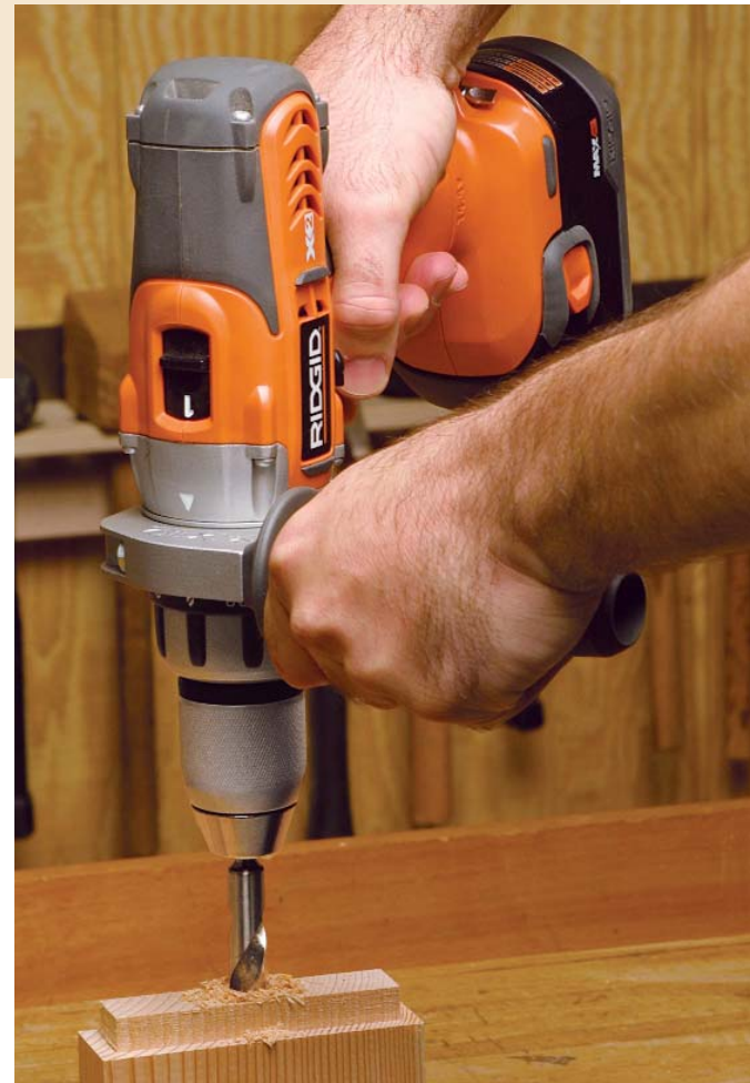
Get a handle on your drill. The Ridgid, as well as the Milwaukee and Bosch, comes with a removable auxiliary handle that provides extra leverage when boring large holes or driving large screws.
