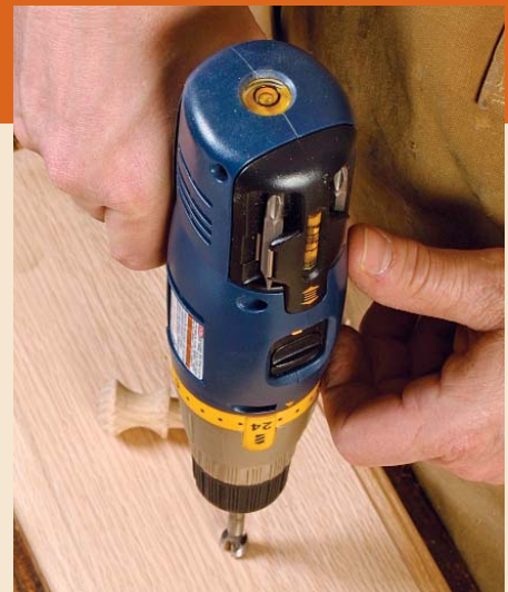
Check for level. The Ryobi drill-driver features two bubble levels, including a bull's-eye level on the back end that helps align the tool 90° for vertical drilling.
