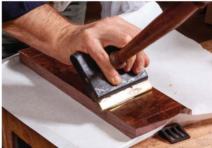
Hammer it down. Use the hammer like a squeegee, starting in the center and pushing bubbles of excess glue and air out at the edges. Keep the edge of the hammer clean with a wet rag.
