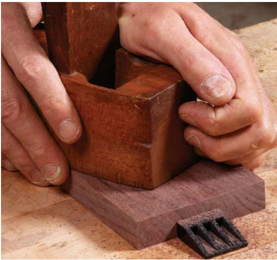
Give the drawer front bite. Latta uses a toothing plane to add texture to the drawer front substrate. It's not essential, but it will help the hide glue hold on better.
