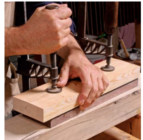
Clamps ensure a good bond. Clamp the veneered drawer front between cauls. Place a sheet of acrylic or waxed paper on top of the veneer to keep the glue from sticking to the cauls. Using clamps isn't strictly required with hammer veneering, but it's quick, easy, and keeps the veneer flat as it dries.
