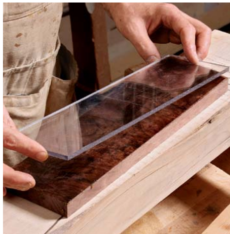
Clamps ensure a good bond. Clamp the veneered drawer front between cauls. Place a sheet of acrylic or waxed paper on top of the veneer to keep the glue from sticking to the cauls. Using clamps isn't strictly required with hammer veneering, but it's quick, easy, and keeps the veneer flat as it dries.
