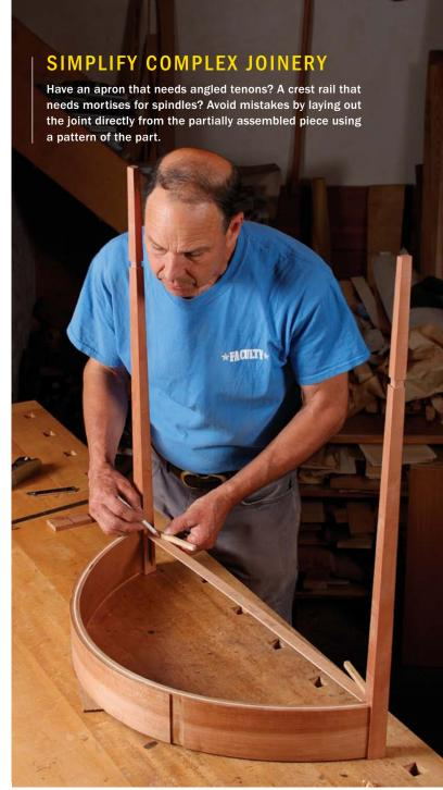
No measurement needed. For angled tenons like those on the back apron of this demilune table, Hack places a pattern of the apron between the back legs and inserts long slip tenons into the mortises. He then traces the exposed part of the tenon onto the pattern to guide his work.
