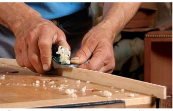
**Refine convex curves with a block plane.** Keep the arc fair. You can square the edge to the face later.
