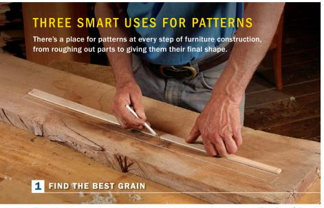
Trace the pattern onto rough lumber to see whether the shape and direction of the grain complements the part's shape. You can also use the pattern to lay out several identical parts (like legs) on a single board before cutting them out.
