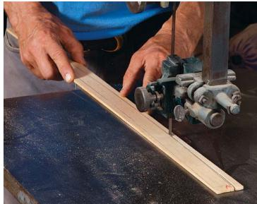
**Use a batten and bandsaw for curves.** A narrow piece of straight-grain basswood, about ½ in. thick, easily bends into a fair curve (left). To hold the ends in place, Hack clamps the batten to a block with a C-clamp, then clamps the block to his bench. Cut the curve as fair as you can (above), so that it's easier to clean it up afterward. A steady hand and feed rate are key.
