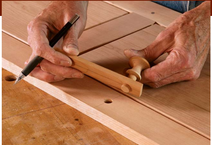
Dry-fit the knob. The hole through the spinner blank should be a snug fit. But the hole in the door stile should be \frac{1}{64} in. oversize to ensure smooth action.
