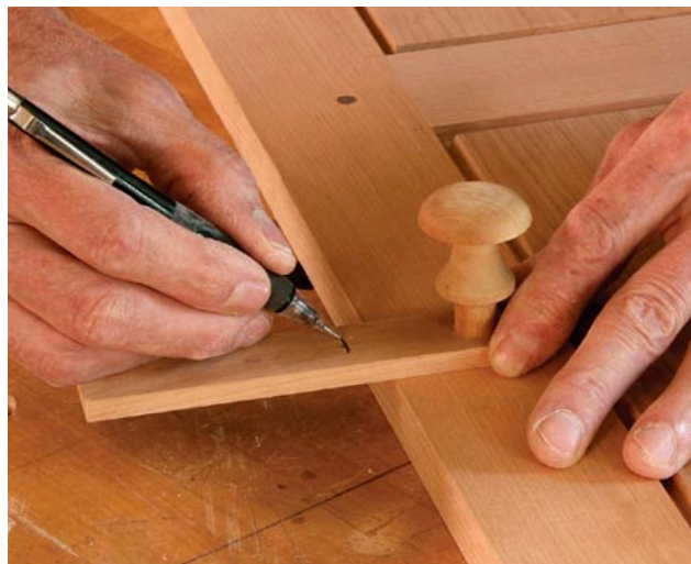
Dry-fit the knob. The hole through the spinner blank should be a snug fit. But the hole in the door stile should be \frac{1}{64} in. oversize to ensure smooth action.
