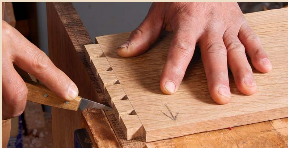
Transfer the tails. Rodríguez cuts the case tails by hand first, then transfers the layout to the sides with a marking knife.
