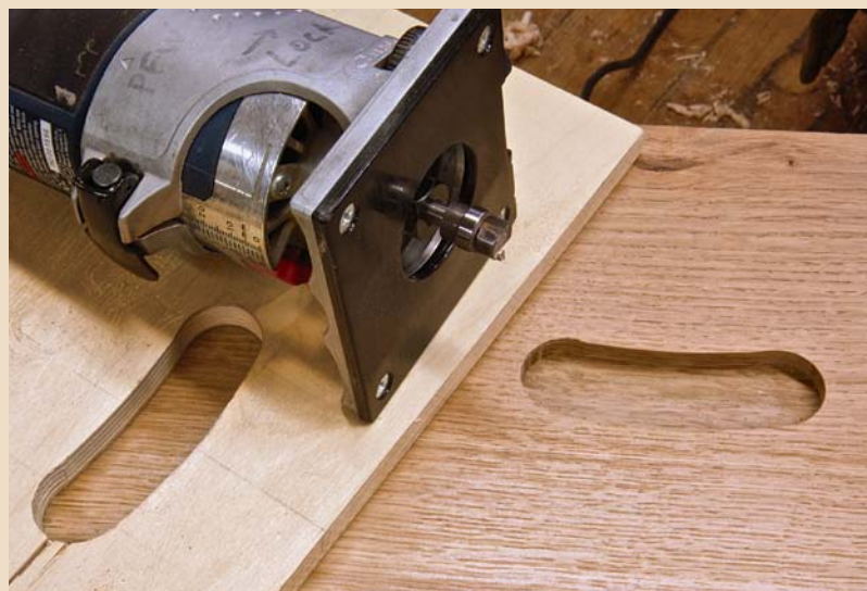
Simple grip. Using a pattern cut out of ½-in. plywood and a router fitted with a bearing-guided ½-in. pattern bit, Rodríguez routes the handholds in the sides of the chest.
