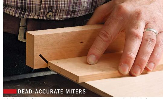
**Bring it to the kerf.** A zero-clearance sled lets you line up the already sized box side with the kerf, no measuring required. Just be sure that the inside of the box is facedown and the upper edge is lined up just right, then clamp down a stop block to keep things in place.
