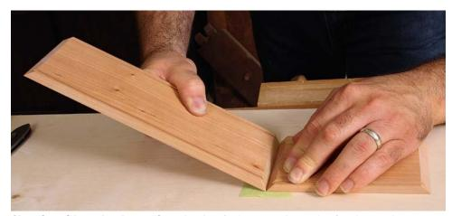
Clamping without the clamps. Once the glue size has properly cured, painter's tape clamps the box together. With tape on a piece laid flat on the bench, place the point of the other piece's mitered edge directly onto the tape. Keeping the two miter tips tight together, lay the piece flat. This ensures the tape will be stretched over the joint, applying even pressure.
