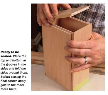
Stretch it tight. To get some clamping pressure on the last corner, Kenney stretches tape over the miter.
