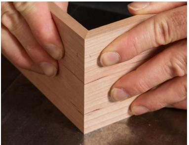
No gap, guaranteed. Kenney's method of cutting for length and then cutting the miter yields perfectly aligned grain across a tight miter.
