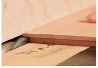
**Cut the tongue.** The bottom is rabbeted at the tablesaw to fit the grooves in the sides. Kenney uses a dado set and an auxiliary fence clamped just above the blade.
