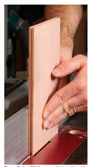
**Groove the top.** With the same settings used to cut the grooves in the box sides, cut a groove around the edge of the box top. It's critical to keep the inside face of the top against the fence to ensure the two grooves mesh perfectly.
