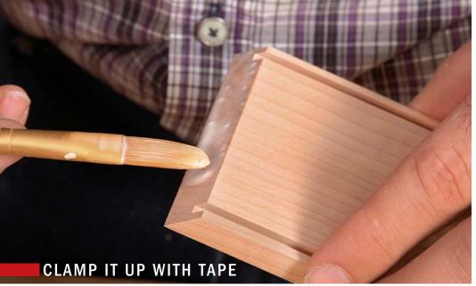
Sized end grain. To help seal the end grain and ensure a good bond at final glue-up, apply glue size, a 50/50 water and Titebond II mix, to the mitered ends. This will fill the end grain and help avoid a glue-starved joint.
