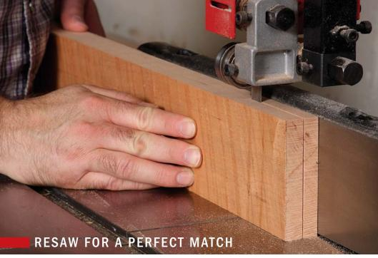
**The match begins.** Joint one face of the 5/4 board. Put the jointed face against the fence and resaw it into two  $\frac{1}{2}$ -in.-thick pieces. Keep track of the inside and outside faces.
