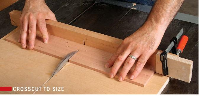
Start with a long side. With a stop block clamped to the sled's fence, cut the first long side to length, keeping the matched grain against the stop. Leave this stop in place to cut the second long side later.
