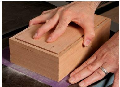
Smooth out the cut. To clean up the machine marks, rub the freshly cut surfaces on a sheet of 180-grit sandpaper on the tablesaw table. To preserve the grain match, apply even pressure and take off only as much as needed.
