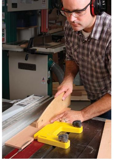
**Remove the overhang.** With the grain aligned, the boards will overhang each other (left). Set up the tablesaw to remove the overhang from the bottom of one board. Then cut both boards to uniform width, referencing their bottoms against the fence.
