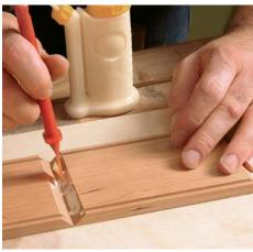
Get to the glue. With all the box sides taped and placed inside-face-up on the bench, carefully spread glue over all the miters except the open ends.
