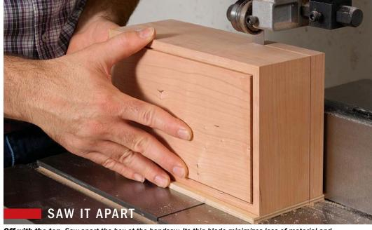
**Off with the top.** Saw apart the box at the bandsaw. Its thin blade minimizes loss of material and gives a tighter match from the lid to the body. Kenney uses the Wood Slicer from Highland Hardware, which is designed for resawing. A piece of thin plywood under the box helps prevent tearout.
