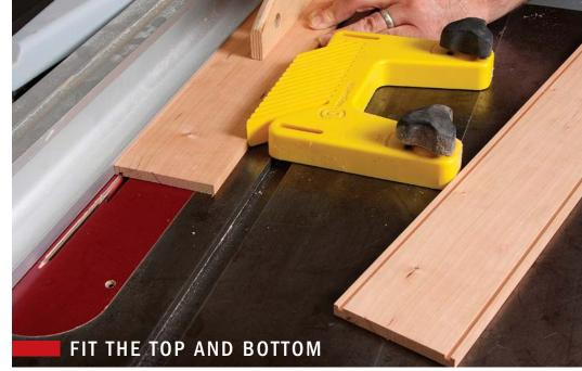
**Cut grooves for the top and bottom.** Each groove is  $^{3}\!/_{6}$  in. deep by  $^{1}\!/_{8}$  in. wide,  $^{1}\!/_{8}$  in. from the edge. Use a featherboard and a push stick to ensure consistency.
