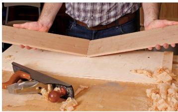
**Slide to align the grain.** After jointing the inside, resawn faces, butt the two boards together with the jointed faces up (above). Slide them up and down until the grain aligns across the pieces (below).
