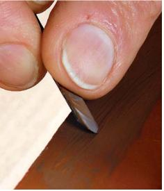
**Hone the back and bevel.** Start with the back, using the edge of a polishing stone (left). Then polish the bevel (right). Don't worry if the bevel has facets. Only the cutting edge matters.
