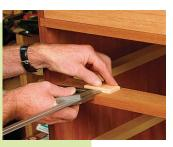
With the ends finished, work on the long edges. Plane away a consistent amount from the top of the drawer. Finally, use a rabbet plane to relieve the bottom edge of the drawer front. Take three or four shavings, leaving the drawer sides resting on the drawer runners but creating a consistent, fine gap all around the drawer front. The lip created by the plane also prevents the bottom edge of the drawer front from catching when the drawer is slid shut.
