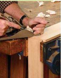
Lightly plane the bottom edges flush with each other (top) and then plane the rear dovetails flush (bottom).
