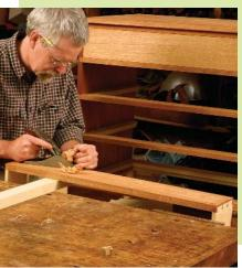
tilted noticeably, you must plane the face to bring it plumb with the case front. Plane very carefully to maintain a flat face.
