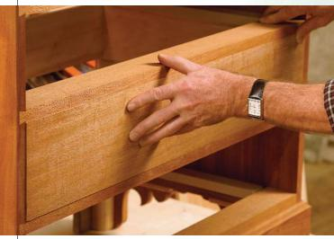
drawer side, it can become too thin at the groove or rabbet that was cut to house the drawer bottom, weakening the construction. If you feel this happening, stop removing material from the back corner and begin planing the drawer face where it protrudes from the case.
