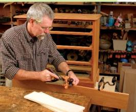
Start with stock  $\frac{4}{16}$  in. too wide. Before planing to fit, check the opening with a straightedge (top). If the dividers or the case is bowed, plane the long edges of the drawer front to match (bottom).
