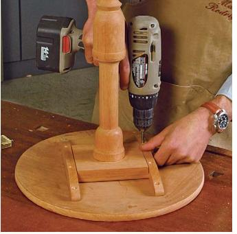
A wedge secures the pivot block. Orient the slot in the tenon perpendicular to the grain of the block to avoid splitting the block as you drive in the wedge.
