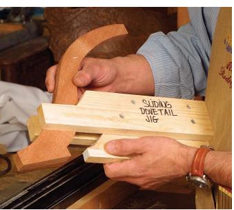
made a jig using my leg template that rides along the router-table fence and holds the leg steady. If you discover that a dovetail doesn't fit right in the column, run it back across the bit and apply more pressure against the fence. It might take off just enough to make the fit easier.
