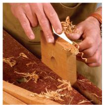
Assemble the pivot block. Glue a separate strip with round tenoned ends into a rabbet cut in the pivot block. Then round the corner of the block to allow the table to tilt properly.
