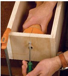
Mount the column in the router jig. First, insert the column into the index block and secure it with a wood screw to keep it from rotating within the block (left). Align the base of the column in the jig using the dimple created by the lathe and hold it in place by tightening the sharpened hex bolt (center). Finally, locate the column for routing by aligning one of the three scribe lines on the index block with the centerline on the jig and fasten it with a screw (right).
