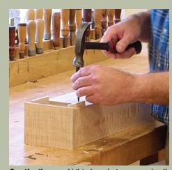
**Gentle glue-up.** Light clamping pressure is all that's needed for the front and back side joints (left). When installing the compartment bottom, use spacers to hold it square while the glue dries, then reinforce with nails set below the surface.
