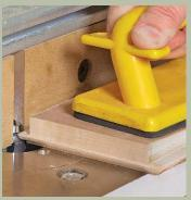
Rout the rabbets and profile. Use a straight bit to rabbet the sides and top of the drawer front (left). Next, use a ¾-in.-radius roundover bit to rout the thumbnail profile on the drawer face (above). Start with the left edge and work in a clockwise direction to remove any crosscut tearout. A zero-clearance fence helps reduce tearout.
