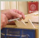
With a scrollsaw and files, prepare the curves. Make relief cuts to the inside corners of the pattern, then cut each sweeping curve to the relief cut (left). Clean up the sawmarks with half-round bastard and smooth files (above).
