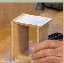
**Pilot holes prevent splitting.** Drill pilot holes after gluing and before nailing the sides to the front. Glue the back to the sides, drill pilot holes (top), and nail (bottom).
