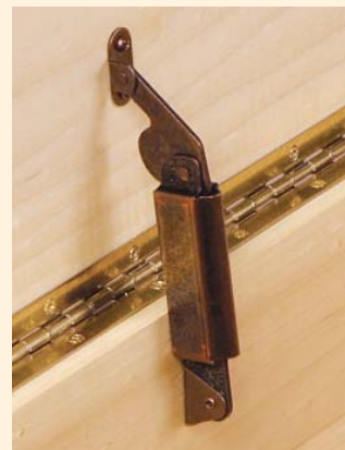
A single center-mounted support. The weight of the lid needs to be matched to the strength of the support's internal spring.
