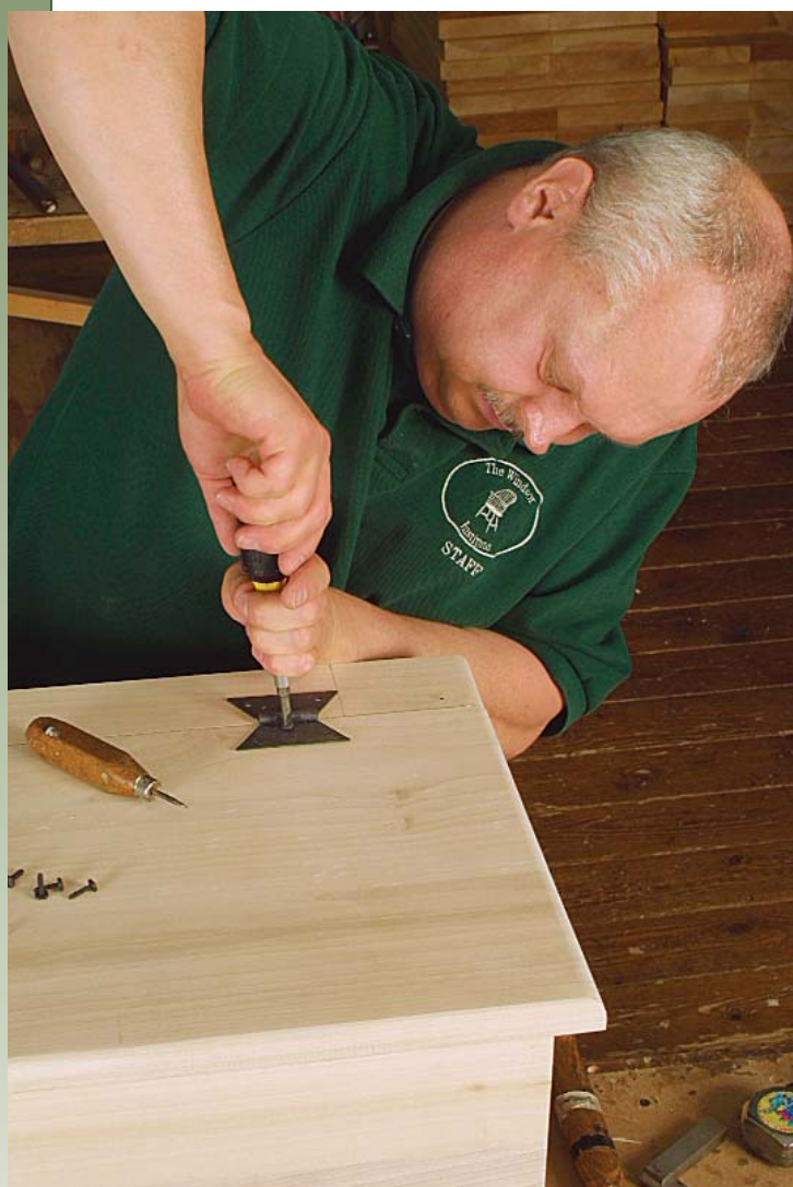
A visible hinge. Butterfly hinges and their close cousin, H hinges, are mounted on top of the lid, which is divided into two parts.
