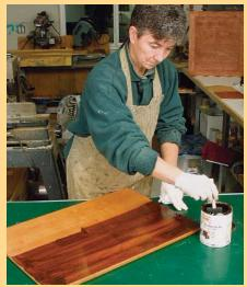
Then brush on a glazing and shading stain. Aim for overall but not uniform coverage. Do the edges last.
