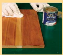
Stain the sapwood. After the coat of varnish has dried, wipe on a coat of gel stain over the lighter area to blend it in (right). If the tone of the gel stain isn't quite right, adjust it by adding some Japan color. Unlike the heartwood, cherry sapwood does not darken with age, so stain the sapwood a little darker than the surrounding wood.
