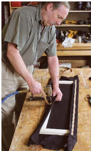
Cloth-covered frame hides speaker. A raw-silk screen conceals the center-channel speaker but doesn't distort the sound.
