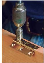
Adjust the countersinks. Use a countersink bit to deepen the holes in the hinge so that the screw heads can sit just below the surface.
