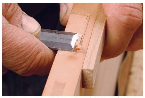
Finish the mortise with sharp chisels. Chop and pare gradually until you reach your layout lines and get a good fit. Save your widest chisels for the final cuts.
