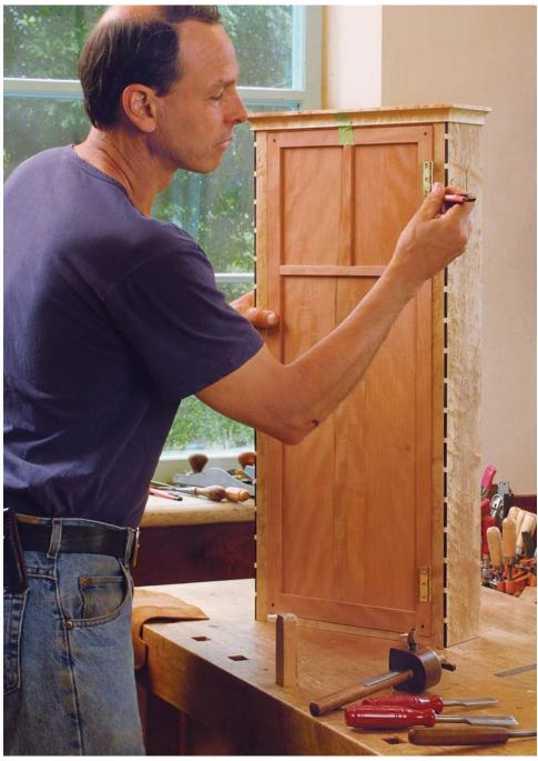
Transfer the hinge locations to the case. With the hinges installed temporarily in the door, shim the door into its final position and use a marking knife for a precise transfer.
