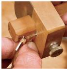
Set the first marking gauge for the width of the hinge. Set it about ½2 in. short of the centerline of the hinge knuckle. The light pencil lines at the end of the mortise indicate where to stop the marking-gauge cut.
