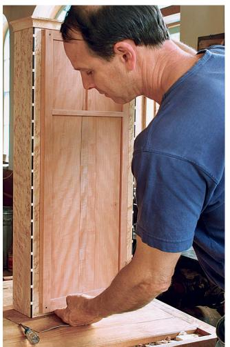
**Cut the mating mortises in** the case and attach the door. Continue to use only one steel screw at this point. Check the fit of the door. If necessary, remove the door and plane it to fit.
