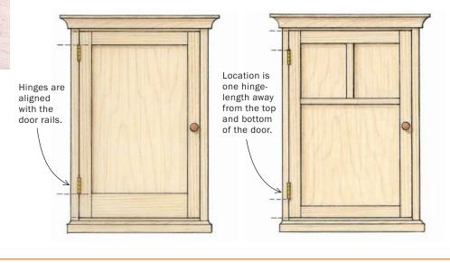
length and width. I prefer fixed-pin hinges over loose pins (the hinge comes apart for lifting off a door easily) because they are stronger with less play in the knuckle.
