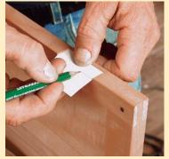
If you've cut too deep. To shim a hinge outward, trim a card to fit into the bottom of the mortise.
