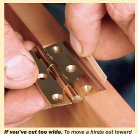
the front of the case, plane a sliver of long-grain wood to fill the gap at the back of the mortise. Glue it in and plane it flush for an invisible repair.
