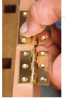
The top hinge is the wrong size for this door. It would leave a fragile sliver of wood at the edge of the mortise. The bottom hinge is a more appropriate size.
