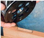
Or rout it out freehand. Set the bit depth to the thinnest part of the hinge and stay clear of the layout lines. For thin doors, you can clamp on an extra board to help support the router base.
