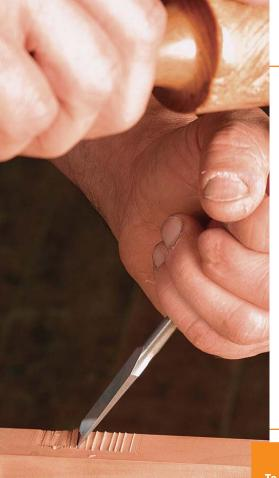
Whether by hand or by machine, the idea here is to clear out the bulk of the mortise while staying clear of your layout lines.
