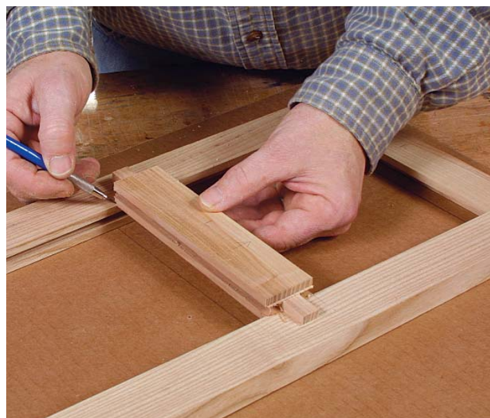
Fit the middle rail. Dry-fit the door frame and fit the middle rail to the piece, using a full-sized drawing as a guide.
