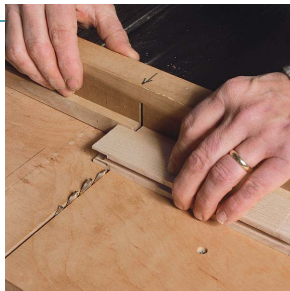
Trim the tapered shoulders on a sled. Nail offcuts from the stiles to a tablesaw sled or miter gauge. The offcuts will provide the correct shoulder angle.
