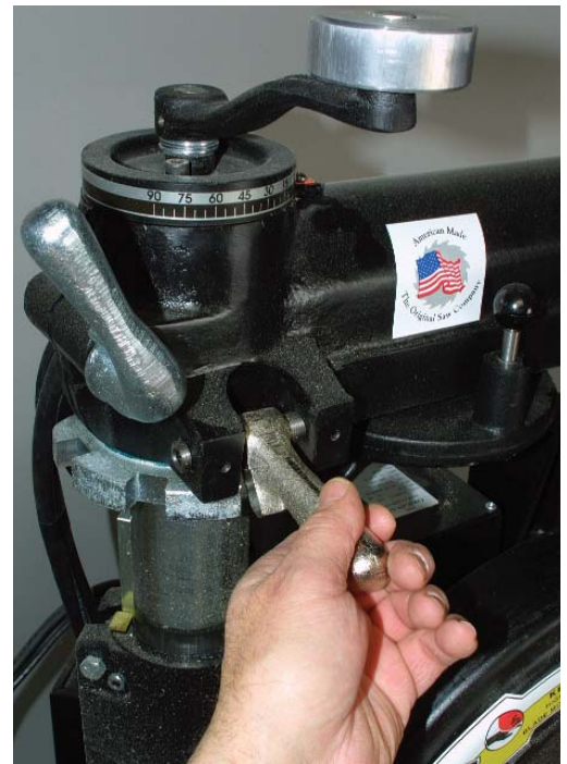
Two handles find the angle and keep it there. The lower handle keys into a notched collar, providing factory-set adjustments for square cuts and 45° miters. The handle at the top tightens the overhead arm onto the column.
