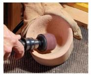
Speedy sanding. Using a Guinevere flex-shaft sanding system with inflatable attachments that conform to the workpiece, Kamerath can smooth any surface quickly.
