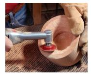
Quick cavity. Kamerath drills out the block with a large Forstner bit. After bandsawing it to an oval, he shapes the interior with a Proxxon mini grinder fitted with a needletoothed carbide carving wheel.
