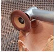
Slots between the drops. Following pencil lines, Kamerath uses the Proxxon grinder to cut notches between the droplets.
