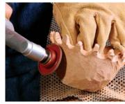
Smoothing time. Using the mini grinder, Kamerath fairs the roughly rounded exterior left by the angle grinder. He follows this step by smoothing the surfaces with the Guinevere sander.
