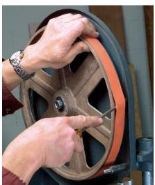
Installing a tire. Stretch the tire over the wheel (top). To even out the tension on the tire, slide a screwdriver between the wheel and tire, then rotate the wheel while holding the screwdriver in one spot (bottom).
