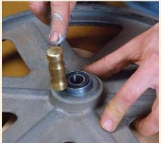
Out with the old, in with the new. A bandsaw wheel has two bearings: Even if only one is failing, they should both be replaced. The wheel bearings must be tapped out with a hammer and punch (left). When installing a new bearing, gently tap it into place using a soft hammer against the outer race (right).
