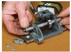
Replace the lower thrust bearing. Remove the nut on the end of the guide rod and slide off the tube to free up the bearing. Clean up everything and, if necessary, slide a new bearing into place.
