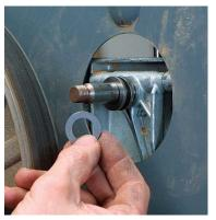
Shim out the upper wheel. If the rims of both wheels aren't touching the straightedge, use shims to bring them into alignment. On Delta saws you can shim the upper wheel; for Taiwanese-made saws, shim the lower wheel.
