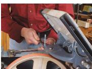
Square the tabletop to the side of the blade. Tip the table and adjust the stop bolt mounted on the trunnion support casting.
