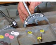
There's only one way to square the table to the back of the blade. You need to insert shims between the table and the trunnions until the blade and the table are aligned. While you have the top off, be sure to clean up and lubricate the trunnions.
