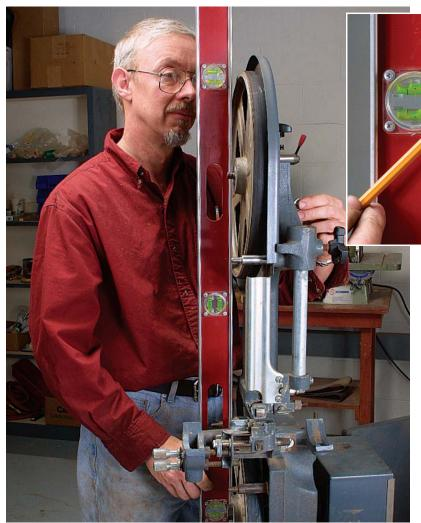
Check the alignment. Begin by placing a long straightedge (White uses a 4-ft. level) across both wheels. Then adjust the tracking mechanism to bring the upper wheel parallel to the straightedge.
