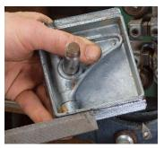
Remove cover and clean up tensioner. With the cover removed (above), it is easy to access the tensioner. Once the tensioner is removed, check to be sure the axle isn't bent, and then file the slides on both sides smooth.
