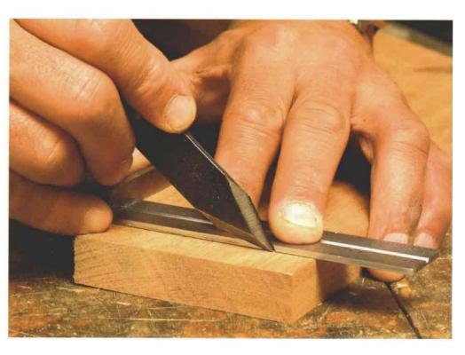
A more advanced use of the marking knife is setting inlay and marquetry into a wood surface. Just as when mortising hinges, accurate work becomes as easy as putting the item in place, cutting a fine line around it and removing the waste.
