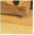
On the shoulders the marking gauge falls short. It tears fibers when used cross-grain and far from its reference edge.
