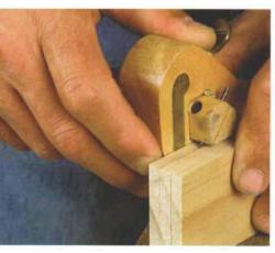
A marking gauge works well for tenon cheeks. The cut is clean because it is with the grain and not far from the fence of the tool.
