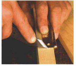
Marking out a hinge mortise. The marking knife adds precision to this operation, too. The line will serve as a starting place for final chisel cuts around the perimeter.
