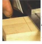
A knife is a better tool for the job. The marking knife leaves a flawless line, regardless of grain direction.
