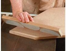
Make a push stick from MDF. Attach sandpaper to the underside of the push stick for a secure gripping surface.
