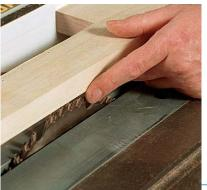
Align the fence flush with the sawblade. Make sure the teeth do not protrude beyond the edge of the fence.
