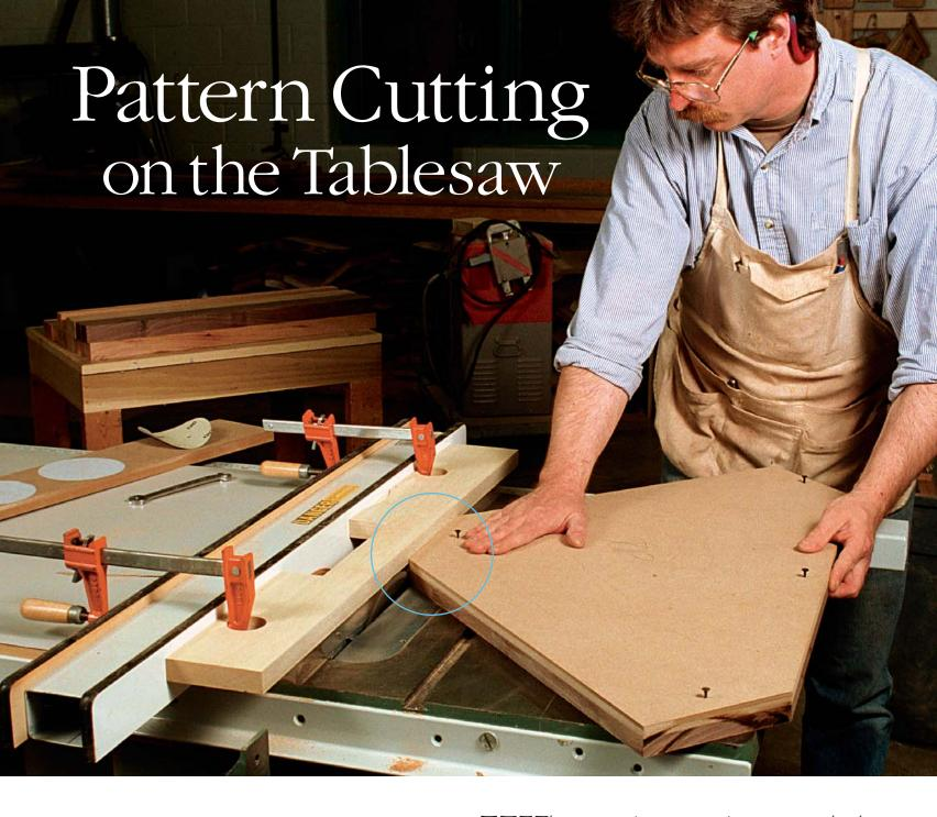
**Duplicate parts** quickly and safely using templates
