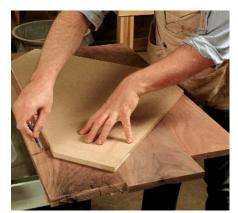
The pattern has two purposes. Trace the shape onto the workpiece for rough-cutting on the bandsaw. Then use it as a template for final trimming on the tablesaw.
