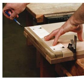
**Use the jig as a tracing guide.** Line it up flush with one stile of the door and mark the area to be trimmed.
