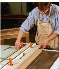
A piece of scrap is used to set the fence height. The auxiliary fence should be ½ in. above the workpiece.
